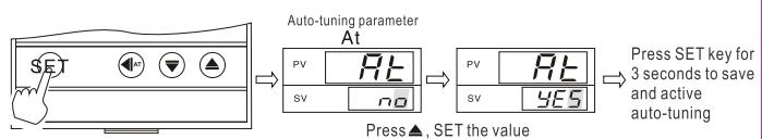
Master controller: the SV value for the auto-tuning process is the SV for the first segment
